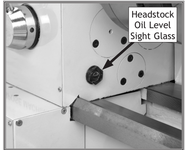
Figure 54. Headstock oil level sight glass.
